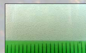
Fig. 6: macro-photograph of the superporous foams containing chitosan and gelatin fixed by crosslinking with transglutaminase.
