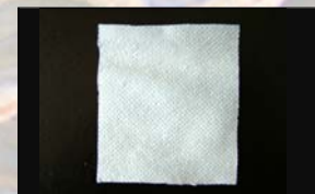
Fig. 3: A sample of a nonwoven fabric prepared from nanofibers composed of the mushroom chitosan (10%) and polyvinylalcohol (90%).
