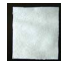
Fig. 3: A sample of a nonwoven fabric prepared from nanofibers composed of fungal chitosan A. niger (10%) and polyvinylalcohol (90%)
