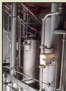
Fig. 2: Propagation station - yeast inoculum preparation
